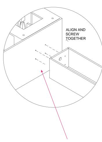
Every connection point CNC set for fast and accurate assembly
